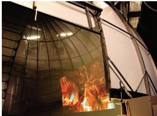
Figure 7. Testing the AlloSphere projection with a single stereo projector with backlighting on to show the screen structure. (Image used with permission of Springer Science+Business Media.)
